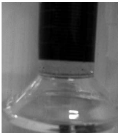
Figure 8. Demulsification results for the heavy crude oil emulsion after 2.5 h at 70 °C with a new composite demulsifier.
